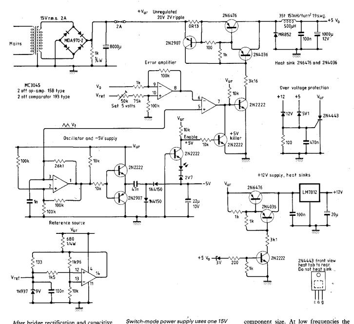
After bridge rectification and capacitive filtering, the 15V r.m.s. transformer output gives approximately 20V. Dynamic rams are sensitive to the sequence in which power is applied to them so the supply had to be designed so that -5V appears first, followed by +5V then +12V.
