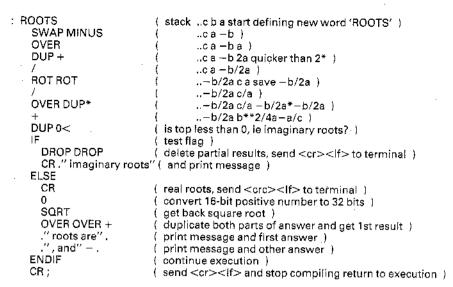
List 7. Forth code used to calculate the roots of a quadratic equation. The stack is represented across the page with the top of the stack at the right.
