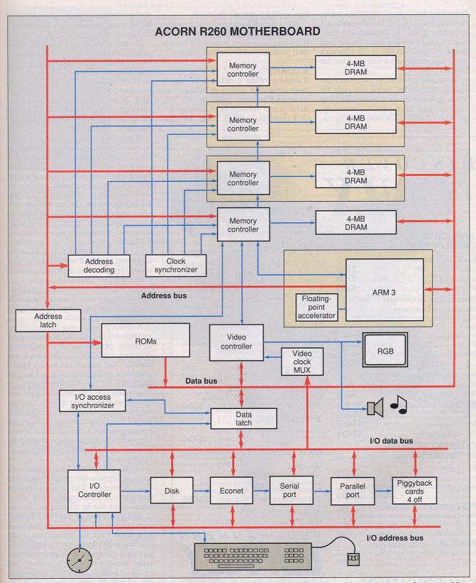
Instead of a CPU, the Acorn R260's motherboard has four proprietary expansion slots. One of them is permanently occupied by the ARM 3 processor. Two of the remaining slots hold 4-MB expansion cards, each containing 4-megabit DRAM chips and its own MEMC chip. The diagram also shows video and I/O circuitry, including four I/O bus slots, serial and parallel ports, thick and thin Ethernet connectors, a socket for stereo sound, and a SCSI connector.
